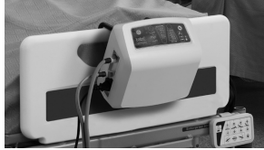
E. Using the bed hooks, hang the control unit on the bed footboard.
