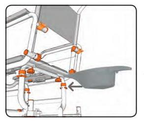
Rotate the chair so that you have easy access to the underside of the seat base.
