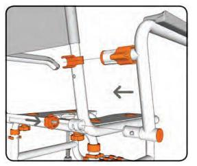
Insert the arm rests into the sockets on the seat base until the clip pin clicks and locates the arm rests in position.
