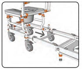
Align the back of your chair with the bridge which is connected to the shower base.
