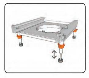
If the tracks are not level horizontally, adjust the height of the shower base until the tracks are level.
