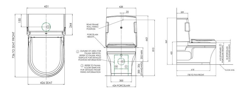
• Safe working load: / • Overall dimensions: 869mm high x 451mm wide x 730mm deep
