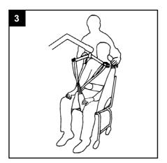
Cross over the leg straps and attach to the spreader bar on the front hooks using the longest loop. Raise the hoist slightly and attach your desired shoulder loop to the rear hooks (a more upright position will be achieved using the shortest loop).
