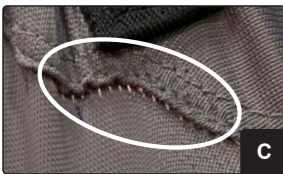
Seam slippage under load (Carer Side)
