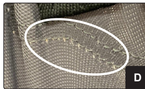
Seam slippage under load (Patient Side)
