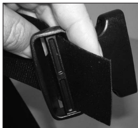
25. Repeat the process 18 to 20 for the other end of the strap. Then feed the strap through the buckle.
