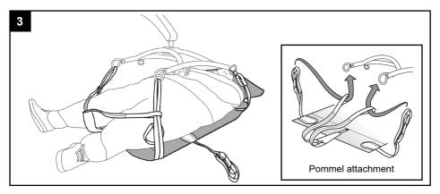
Move the lift into position above the client, keeping the cradle hooks away from the client's face. Attach the shoulder and leg straps to the respective front and rear hooks on the cradle, ensuring to feed each leg strap through the corresponding pommel loop (see diagram above). Adjust the head support to suit client comfort.
