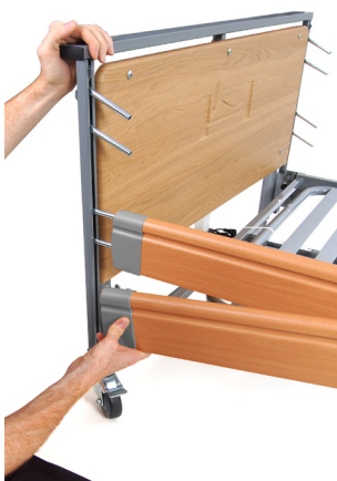
Push the end panel back towards the mattress base and place the base onto the mounting lug. Fix both the spring-loaded catches securely in place.
