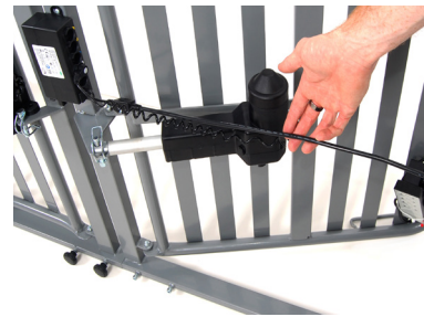
Ensure the power cable runs underneath the actuator
