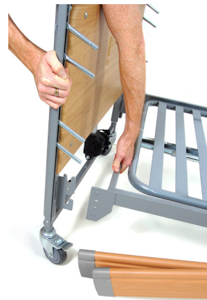
Lift one corner of the mattress base slightly. Pull back the bed end panel with mounting lug
