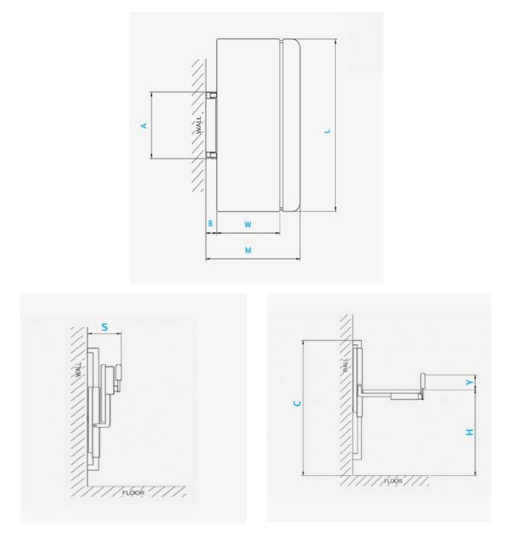
The diagram above shows the relevant dimensional sizes of the Changing Bench. Below *(Table 3)* is a table containing the dimensions of each size. All dimensions are in mm unless otherwise specified.
