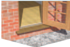
Wood/Level Access Door Threshold
