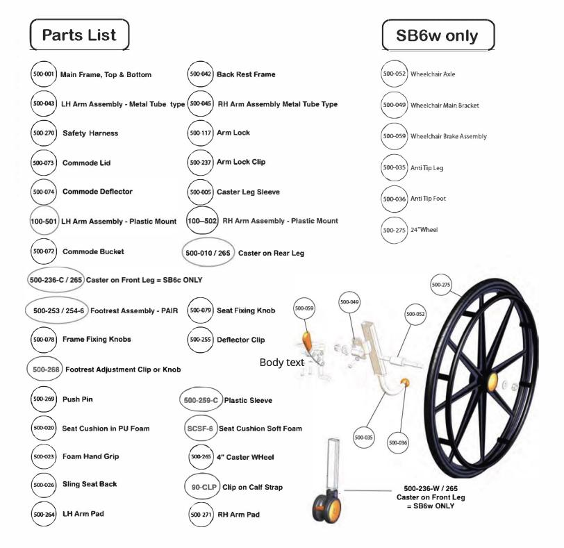
This Universal Parts List for SB6c and SB6w includes original and updated design components. Check the exploded parts diagram to obtain the correct part for your chair. if unsure contact your supplier.
