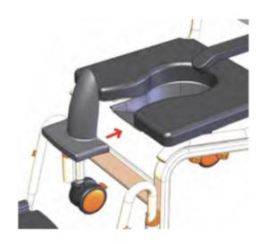
Adjust the Seat height. To raise of lower the seat height depress the push pin in the caster leg and move the leg up or down.
