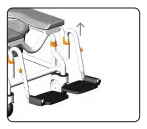
To swing the footrest out of the way simply lift the leg out of the slot and spin the leg away.
