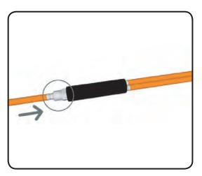
Check to ensure that the cable adjustor is screwed all the way in as shown.
