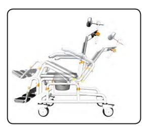
While squeezing the brake handle the chair can be returned to the upright position.
