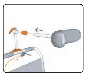
To attach the neck rest, insert the plastic sleeve into the neck rest height adjustment tube.
