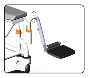
With the footrest in the swing-away position the footrest can easily be removed.
