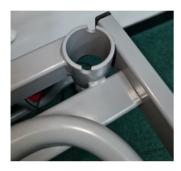
8. Ensure the lifting pole is pointing towards the centre of the mattress platform and the lugs on the lifting pole are fully located in the slots on the socket.
