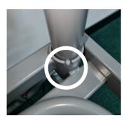
6. Check the strap on the triangle is secure and routed through the buckle correctly
